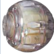
Figure 1: Final production version of the ADC phantom. A clear polycarbonate shell provides waterproofness, strength, and transparency to easily assess ice-water levels and the presence of air bubbles. Silicone susceptibility-matching plugs covering the equatorial fasteners mitigate image artifacts, facilitating image analysis.
